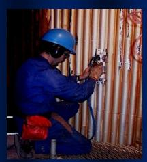
E-PIT<sup>TM</sup> Tools are designed to inspect tubes & pipes from the outside surface to detect internal (ID) & external (OD) defects. This is useful for situations where a pipe must be inspected before it is taken out of service.
